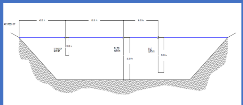
Figure 3. Cross section of turbidity control system
